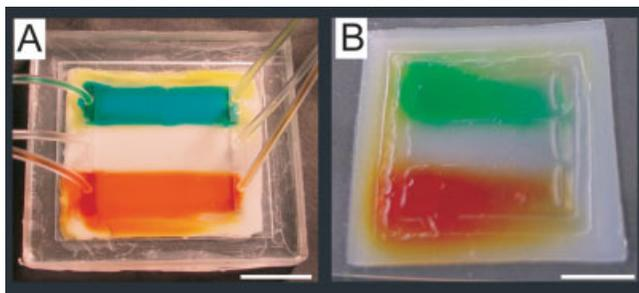
**Figure 8.** Patterned delivery of solutes. (A) Top view of AWD acting on a calcium alginate substrate after operation for 120 min to deliver three separate solutes. (B) Top view of corresponding patterned substrate. The scale bars in both images correspond to 1 cm. [Color figure can be viewed in the online issue, which is available at [www.interscience.wiley.com](http://www.interscience.wiley.com).]
